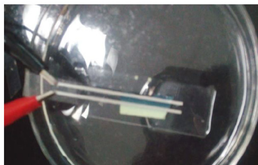
Image 1: Change in colour in presence of electric charge in WO_3
